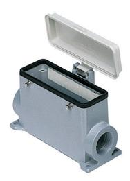
Surface mounting housing, 830V series, with 4 pegs, M32 x 2 cable entry, size "104.27", high construction, with plastic cover
