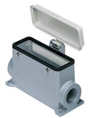
Surface mounting housing, 830V series, with 4 pegs, Pg29 x 2 cable entry, size "104.27", high construction, with plastic cover
