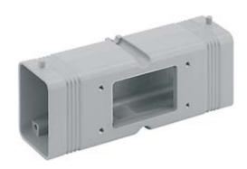
T-BOX coupler, for 2 hoods size "44.27" with lever and gasket and one Bulkhead mounting housing size "44.27"
