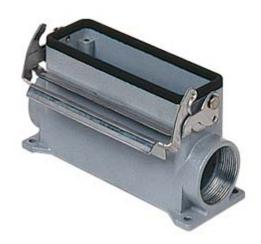
Surface mounting housing, V-TYPE series, with 1 lever, Pg21 x 2 cable entry, size "104.27", high construction
