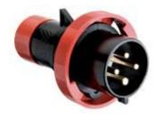
Mobile plug, PLUSO HEAVY DUTY series, 3 poles + PE, 6 h (red), 32 A, 380  $\div$  415 V, straight
