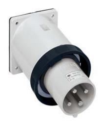
Flush-mounting plug, PLUSO series, 2 poles + PE, 7 h (black), 63 A, 480  $\div$  500 V
