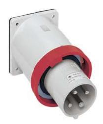
Flush-mounting plug, PLUSO series, 3 poles + PE, 11 h (red), 63 A, 440  $\div$  460 V
