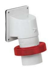
Flush-mounting plug, PLUSO series, 3 poles + PE, 11 h (red), 32 A, 440  $\div$  460 V
