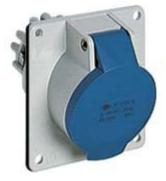
Flush-mounting socket outlet, PLUSO series, 3 poles + PE, 9 h (blue), 32 A, 200 ÷ 250 V, inclined
