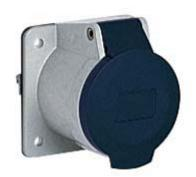
Flush-mounting socket outlet, PLUSO series, 3 poles + N + PE, 5 h (black), 32 A,  $347/600 \div 400/690$  V, straight
