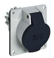
Flush-mounting socket outlet, PLUSO series, 3 poles + N + PE, 5 h (black), 32 A,  $347/600 \div 400/690$  V, inclined
