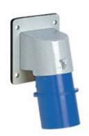
Flush-mounting plug, PLUSO series, 3 poles + N + PE, 9 h (blue), 16 A, 120/208  $\div$  144/250 V
