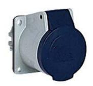
Flush-mounting socket outlet, PLUSO series, 2 poles + PE, 7 h (black), 16 A,  $480 \div 500 \text{ V}$ , straight
