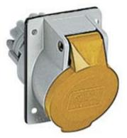
Flush-mounting socket outlet, PLUSO series, 3 poles + N + PE, 4 h (yellow), 16 A, 57/100  $\div$  75/130 V, inclined
