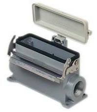
Surface mounting housing, V-TYPE series, with 1 lever, M25 cable entry, size "104.27", with plastic cover
