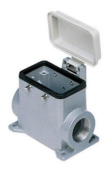
Surface mounting housing, C-TYPE series, with 4 pegs, M40 cable entry, size "57.27", high construction, with plastic cover
