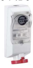
Interlocked switched socket-outlet, IB6 series, 3 poles + PE, 6 h (red), 63 A,  $380 \div 415$  V, sectionable fuse carrier 22 x 58 mm
