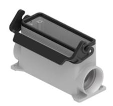
Surface mounting housing, JEI\$-P series, with 1 lever, M32 x 2 cable entry, size 104.27, high construction
