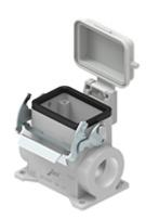
Surface mounting housing, JEI®-V series, with 1 lever, Pg16 x 2 cable entry, size "44.27", high construction, with plastic cover
