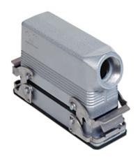
Complete connector, JNZ series, composed of 2 screw terminal connection inserts with 10 poles + PE, and bulkhead mounting housing with 2 levers and hood with side cable entry
