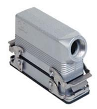
Complete connector, CSZ series, composed of 2 spring terminal connection inserts with 24 poles + PE, and bulkhead mounting housing with 2 levers and hood with side cable entry
