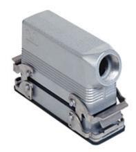
Complete connector, CSZ series, composed of 2 spring terminal connection inserts with 10 poles + PE, and bulkhead mounting housing with 2 levers and hood with side cable entry
