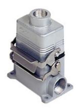
Complete connector, CSZ series, composed of 2 spring terminal connection inserts with 6 poles + PE, and surface mounting housing with 1 lever and hood with top cable entry
