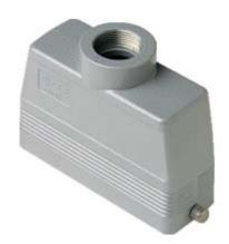
Hood, 830V series, with 1 lever, Pg21 top cable entry, size "104.27", high construction
