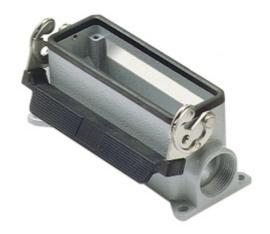
Surface mounting housing, 830V series, with 1 lever, Pg21 cable entry, size "104.27", high construction
