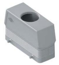
Hood, C-TYPE series, with 4 pegs, Pg21 top cable entry without adapter, size "104.27", high construction
