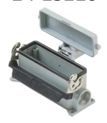
Surface mounting housing, C-TYPE series, with 1 lever, Pg29 x 2 cable entry, size "104.27", high construction, with metal cover
