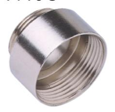
Reduction nipple, with gasket, male M 40 / female M 50 threading
